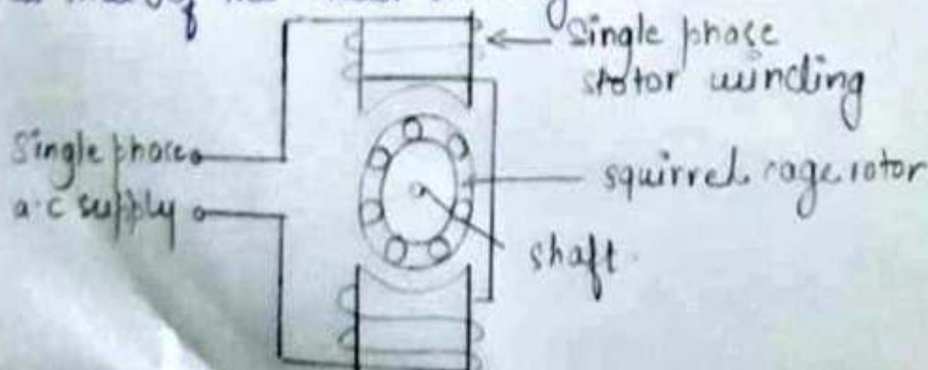
\* Working principle of Single phase Induction Motors:
