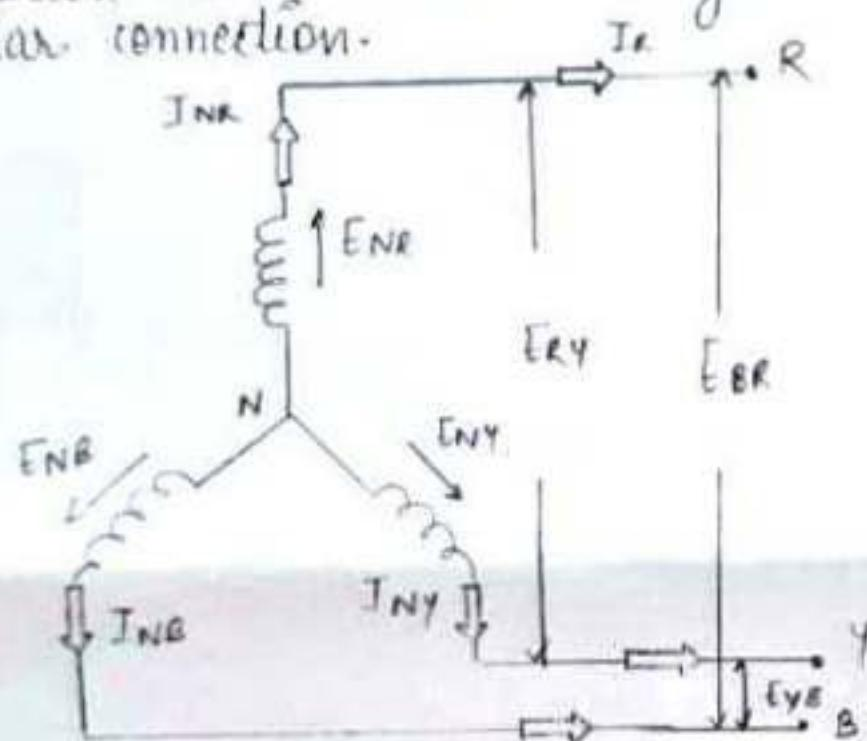
As the system is balanced, balanced system means that in all three phases, R, Y and B, the equal amount of current flows through them. Therefore, the three voltages  $E_{NR}$ ,  $E_{NY}$  and  $E_{NB}$  are equal in magnitude but displaced from one another by  $120^\circ$  electrical.
