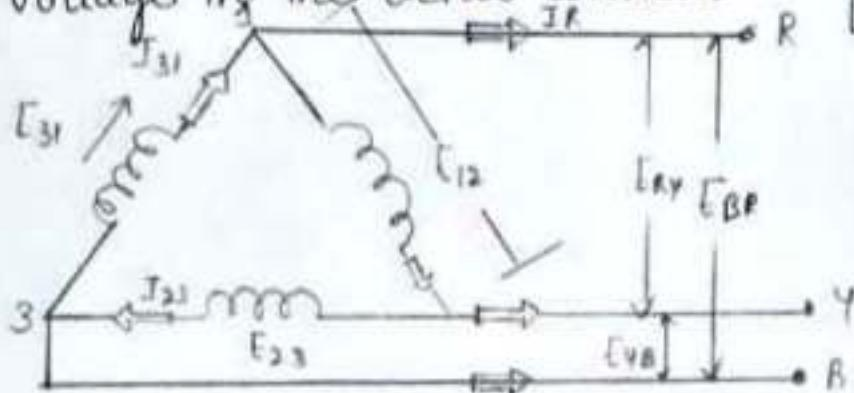
It is clear from the fig that the voltage across terminals 1 and 3 is the same as across the terminal R and Y. Therefore,
