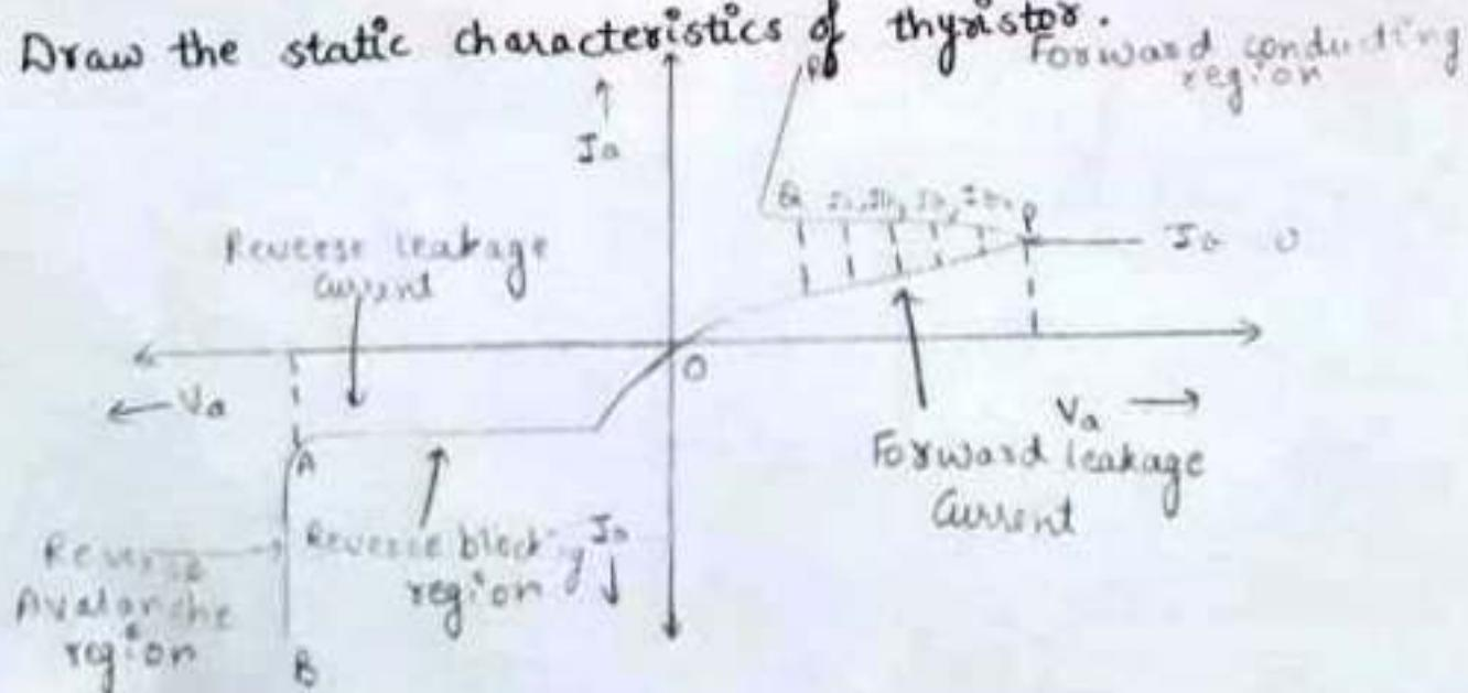
Thyristor are current operating devices, a small Gate current controls a larger Anode current.
